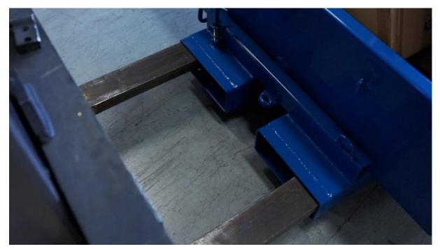
3. Tighten the built-in fork locking for safe handling.
