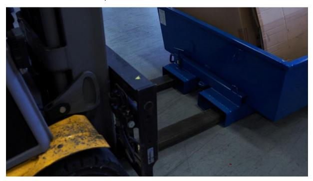
2. Spread the forks outward so that the forks clamp.
