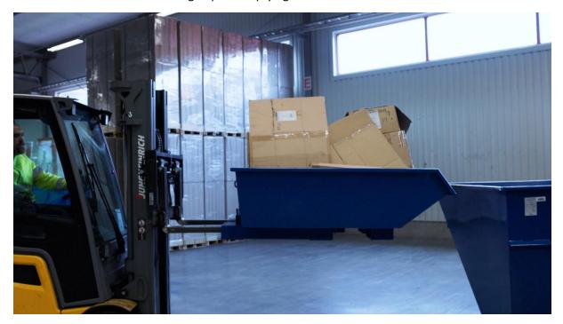
5. Drive carefully towards the edge of the container you are emptying into. Lower the tilting skip over the endge.
