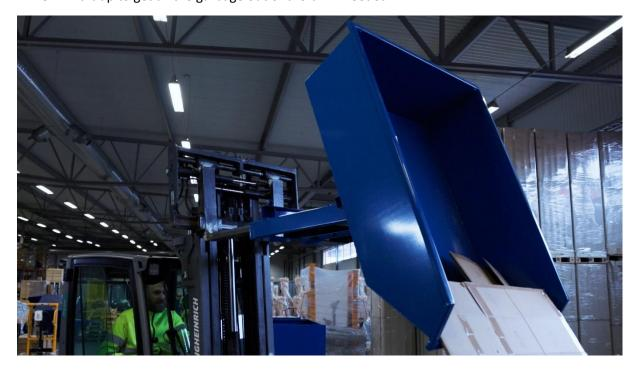
9. When empty, lift it back and lower it to the ground while slowly driving backwards so that the bin tilts back on the undercarriage again.
